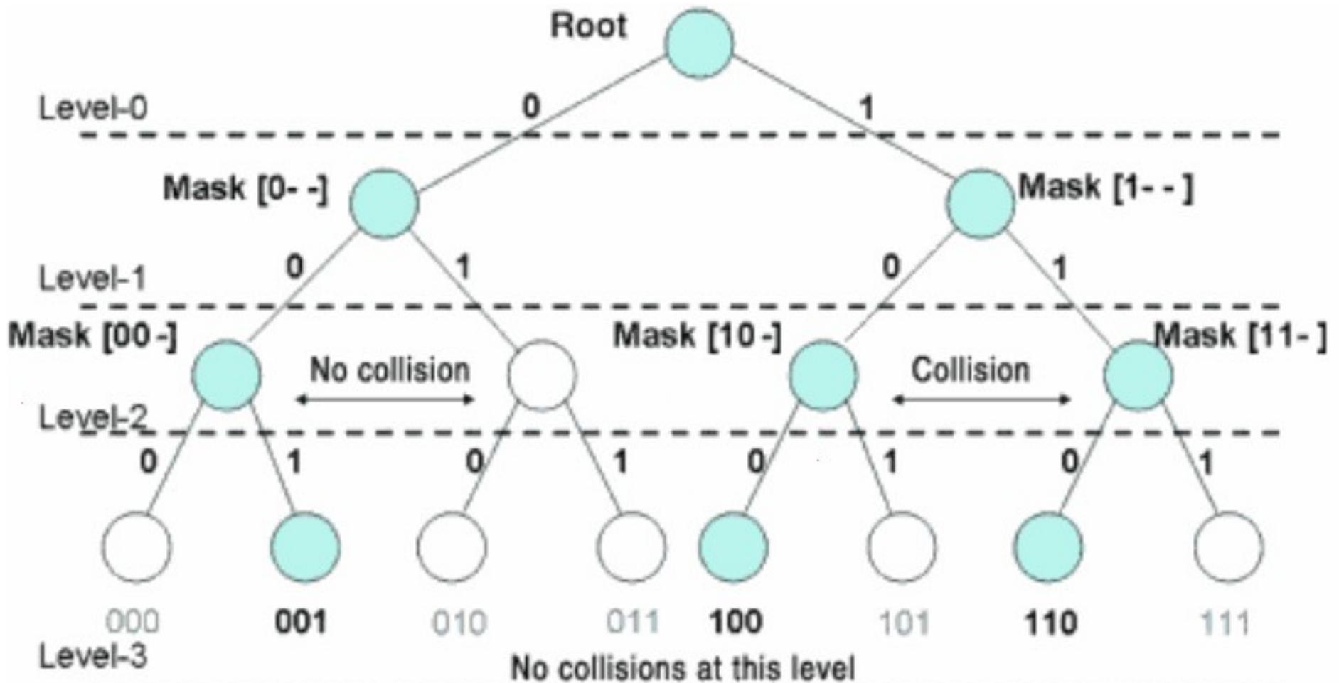
Example using 3-bit tag IDs. Three tags 001, 100, and 110 are in bold
