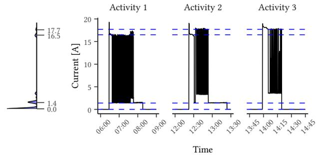
Figure 5: SolderingOven: Current during periods of activity.
