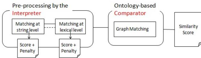
**Fig. 9.** Ontology-based data matching model
